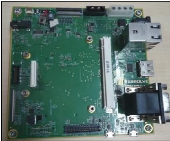
Fig 4: Photograph of Carrier Board
